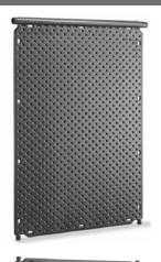
1000 OKU absorber with integrated collecting pipe d 40 mm and two hose couplings d 25 mm Dimension 1320 mm x 820 mm Collecting area 1.08 m<sup>2</sup>
