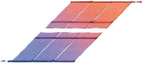
The water of the swimming pool can flow through the oku absorbers in either direction, so they can be mounted both lengthwise and side by side. The individual rows of absorbers are connected on a Tichelmann principle (same routes for each row). It is not advisable to connect more than seven absorbers in series.
